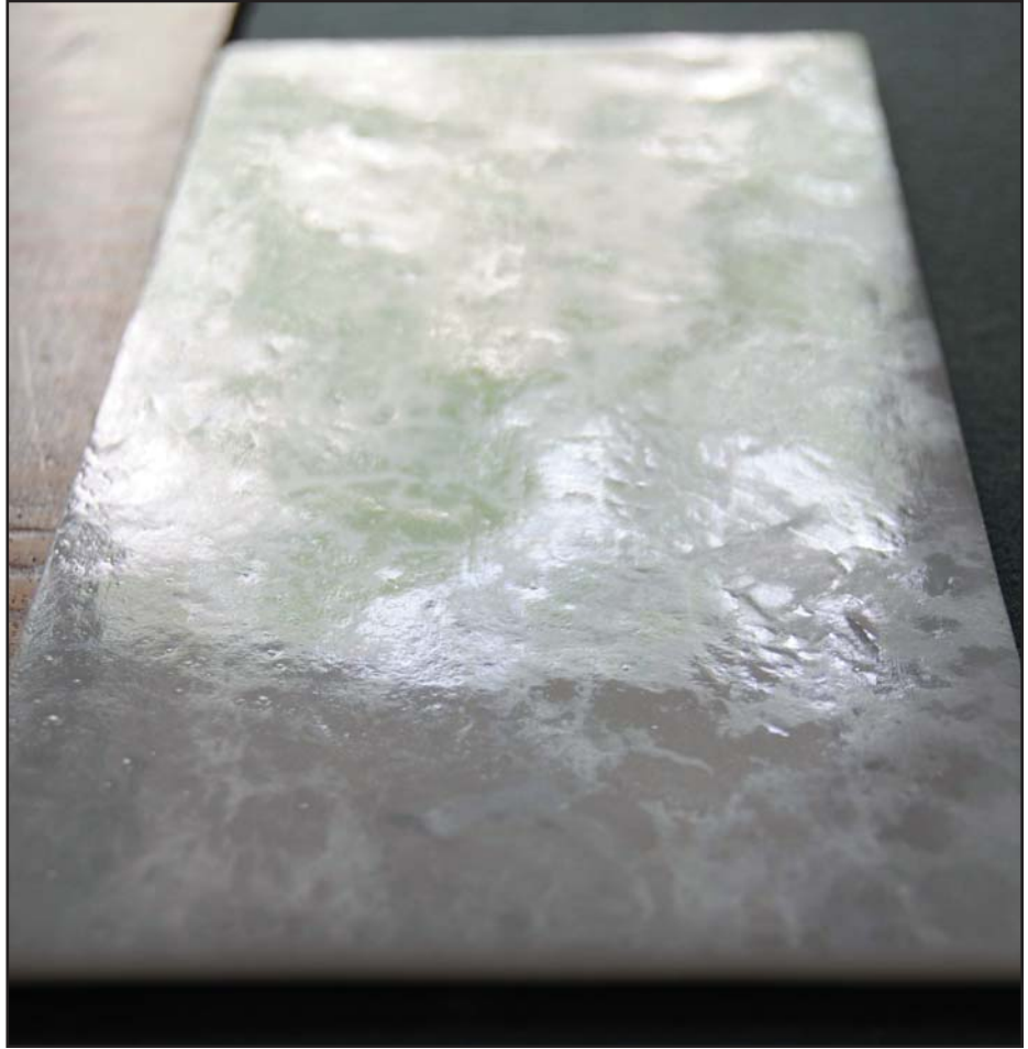
Opalescent whites can tend to devitrify during the firing process, especially on the kiln shelf side.
